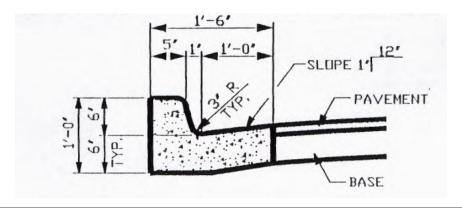
Transition from 2'- 6" Valley Gutter to 1' - 6" Curb and Gutter
